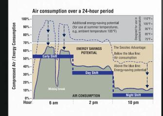
The graph shows a typical compressed air consumption profile. Secotec dryers save energy because the refrigerant system is shut down during breaks, periods of low demand, and downtime; the control system operates without fixed run-on periods. The integrated thermal mass ensures that the system is always ready for operation.
