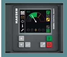
TE and TF models include Sigma Control Smart, a micro-processor based controller which controls the thermal storage process. It has an alarm and service message memory, as well as remote on/off control capability. An optional Modbus TCP interface for connecting to a master control system is also available.
